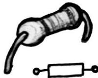
[Resistors](#) work often same way as wires, except that they don't conduct as much current, i.e. they have a resistance. A bigger resistance means less current and vice versa. Resistance is marked to the body of a resistor with color codes commonly found online. Typical resistances range from hundreds of ohms ( $\Omega$ ) to millions of ohms (megaohm,  $M\Omega$ ), most used being kilo-ohms ( $k\Omega$ ).
