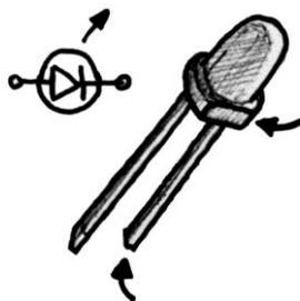
[LED](#) is a diode that starts to emit light when conducting. Since LEDs need only a little current, they are becoming more and more the standard in lighting, and they have been around for decades as indicators. LEDs, similar to diodes and zeners have got a threshold voltage that's different for different colors of leds. A red led typically lights at less than two volts, while green leds need something like 4 volts.
