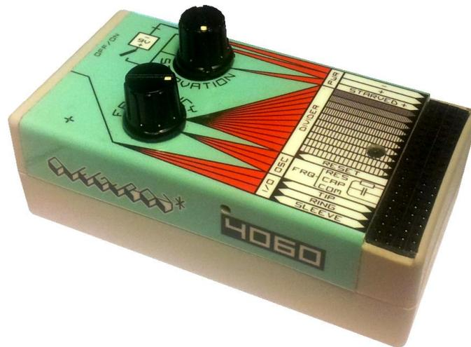
Olegtron\* 4060 is a compact oscillator/divider box capable of creating unique signals and sequences through a revolutionary programming method of sticking components to it's patchboard!
